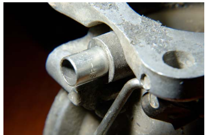
Figure 6 Close up of test fitting of the new bushing
