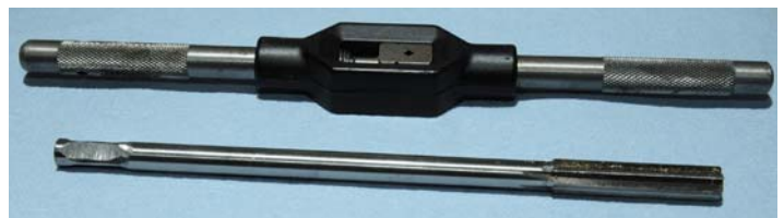
Figure 1 Alvord-Polk Tool Chucking Reamer, Straight flutes (spiral is good too), and a tap handle. Notice the square cross-section ground near the end of the shaft of the reamer to accommodate the tap handle. A great supplier is MSC Industrial Supply ( www1.mscdirect.com/cgi/nnsrbr )
