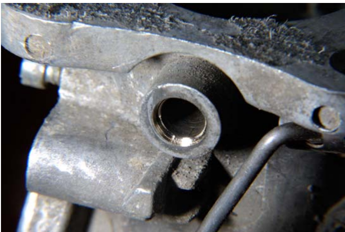
Figure 5 Close up of the initial reaming of the original bushing
