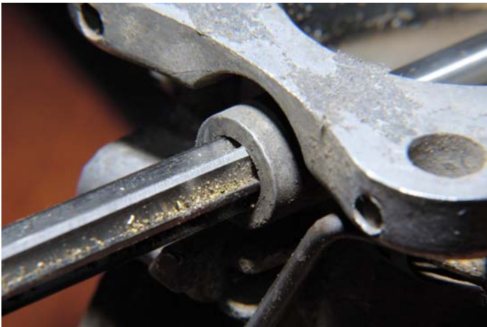
Figure 4 Close up of the reamer in position.
