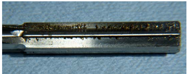
Figure 2 Close-up of the flutes of the reamer with the back-cutting modification.
